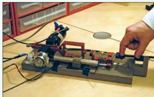
Close-up view of the master (the operator interface). The force is measured as close to the finger as possible. The system also measures the position and speed of the motor.
