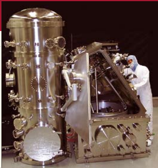
Test set-up of an extreme UV exposure system developed by Sandia National Laboratories. The heavy stainless steel structure is needed to ensure sufficient stability of the writing system and structural integrity for working in vacuum.
