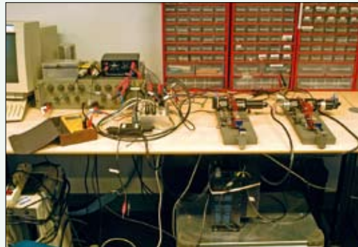
The experimental set-up used at the Delft Biorobotics Laboratory to test the soft/hard theory. On the right is the master, with the slave to the left of it.
