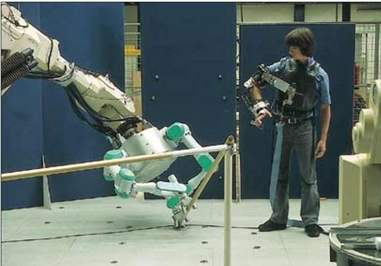
The Eurobot is controlled by an astronaut from inside the ISS. Force feedback would be a useful feature to prevent the Eurobot damaging the ISS. For this purpose, TU Delft doctorate student André Schiele is working at ESTEC to develop an exoskeleton that will enable astronauts to operate the Eurobot while providing force feedback from the robot to the astronaut.
