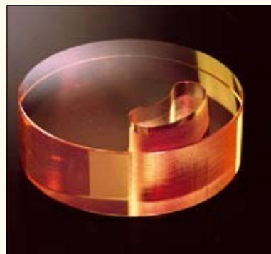
Example of an extreme UV mirror substrate, made from Zerodur. This type of glass, with its characteristic yellow colour, is designed to minimise the changes in shape and size due to temperature changes. The reflective coating is deposited onto the practically transparent material in several layers.
